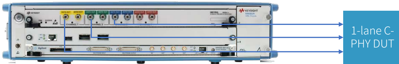
Alternative setup: M8195A, 2 slot frame, embedded Controller
